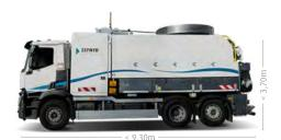
The 3 tank design of the *ZEPHYR* combination unit allows the operator to perform different kinds of interventions on the same trip (septic tanks, municipal networks and grease traps).
